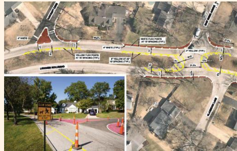
The City of Kirkwood, MO, installed quick build safety improvements as an engagement activity during the Vision Zero Action Plan development process.
